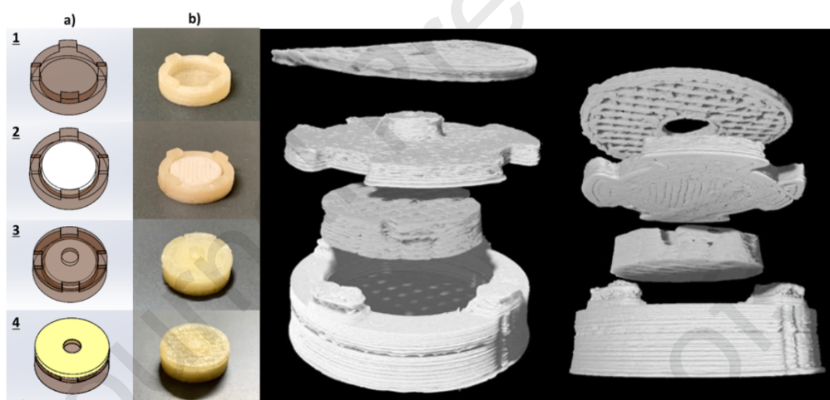
Fig. 6. (a) Design, (b) 3D printed and (c) X-ray CT rendering of the 3D printed compartments of the solid dosage form. From left to right, bottom compartment of the placebo section, top compartment of the placebo section, caffeine compartment and Melatonin compartment. Reprinted with permission from (Ghanizadeh Tabriz et al., 2023).
