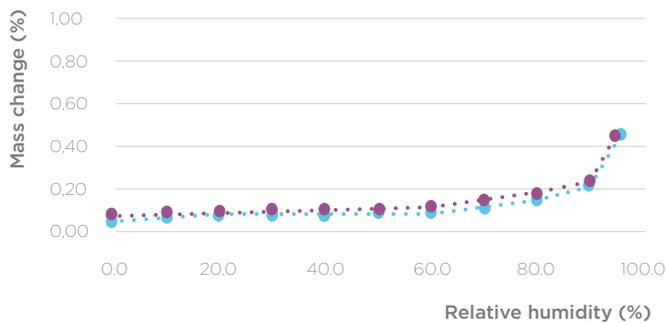
Lactalpha 100 sorption isotherm at 25°C, measured by SPSx-1µ vapor sorption analyzer.
