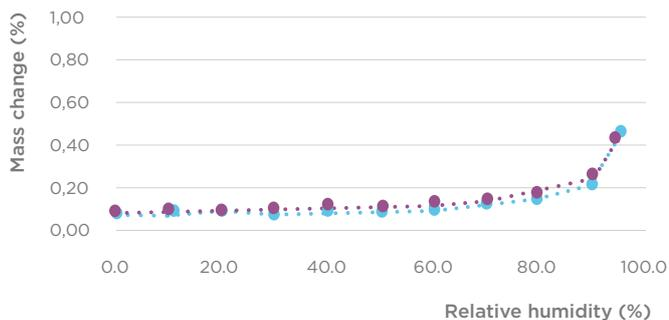
Lactalpha 150 sorption isotherm at 25°C, measured by SPSx-1µ vapor sorption analyzer.
