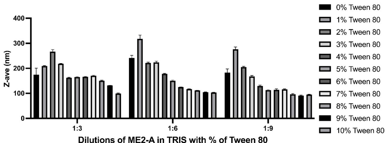
**Figure 1.** Mean droplet size ME3-A, with different dilutions of ME2-A in TRIS and different amounts of Tween<sup>®</sup> 80. Values are reported as mean of at least 3 measurements  $\pm$  SD.
