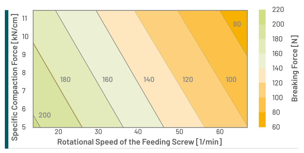
Fig. 3 Contourplot of the breaking force [N] of tablets (relating to a tableting compaction force of 10 kN). RCDG material of SMCC:DCP was produced at a constant roll speed (8 min<sup>-1</sup>), varying specific compaction forces and screw speeds
