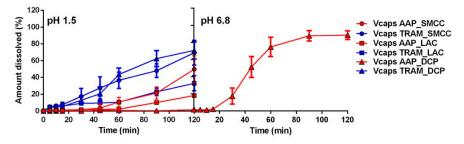
**Figure 7.** Release profiles of Vcaps capsules containing AAP or Tram as API and silicified microcrystalline cellulose (SMCC), anhydrous lactose (LAC), and anhydrous dibasic calcium phosphate (DCP) as filler.
