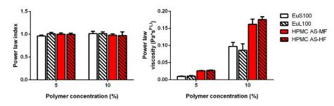
**Figure 1.** Effect of polymer type and concentration on the power law index (**left panel**) and the power law viscosity (**right panel**) as determined from a power law modeling of the viscometry data.
