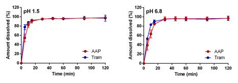
Figure 2. Release profiles of uncoated capsules containing AAP or Tram at pH 1.5 and 6.8.
