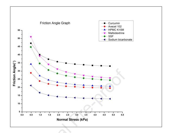
Figure 2. Wall friction angle of curcumin and excipients results obtained by five-pointpoint data set with powder flow software.
