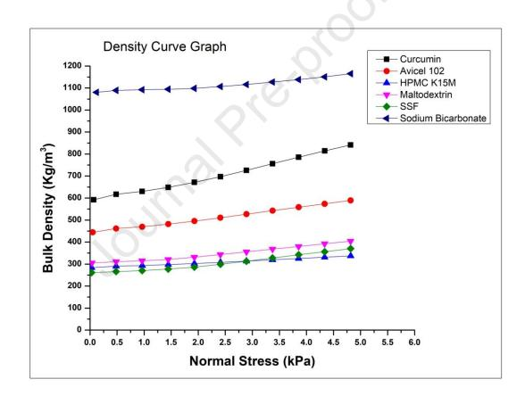
**Figure 3.** Bulk density of drug and excipients results obtained by five-point point data
