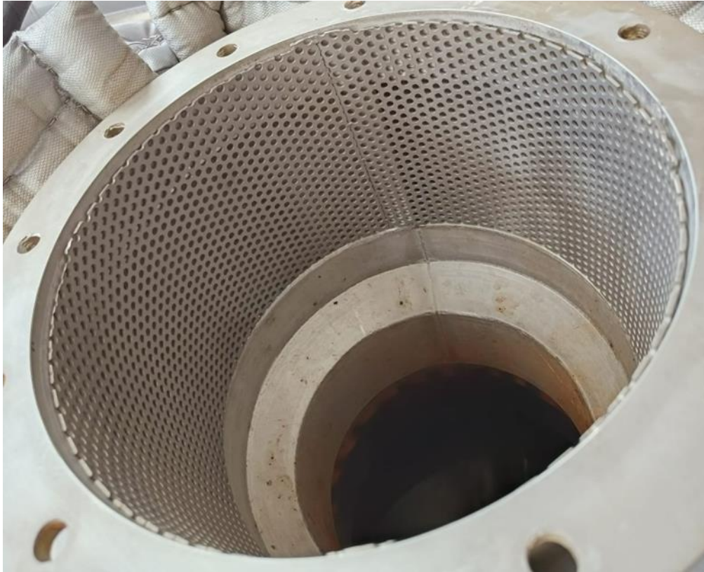
Figure A. 1: Detailed picture from the perforated basket inserted in the air distributor.
