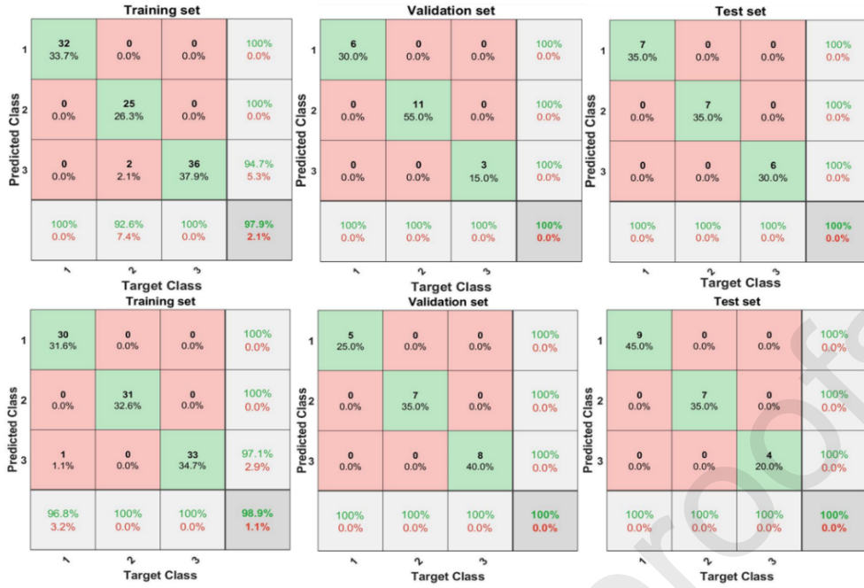
Figure 9. The confusion matrixes for training, validation, and test sets for VIS (first row) and UV (second row) images (1. group: MLX_{25\mu m} , 2. group: MLX_{176\mu m}^{Acetone} , 3. group: MLX_{176\mu m}^{Acetone} + MLX_{25\mu m} )
