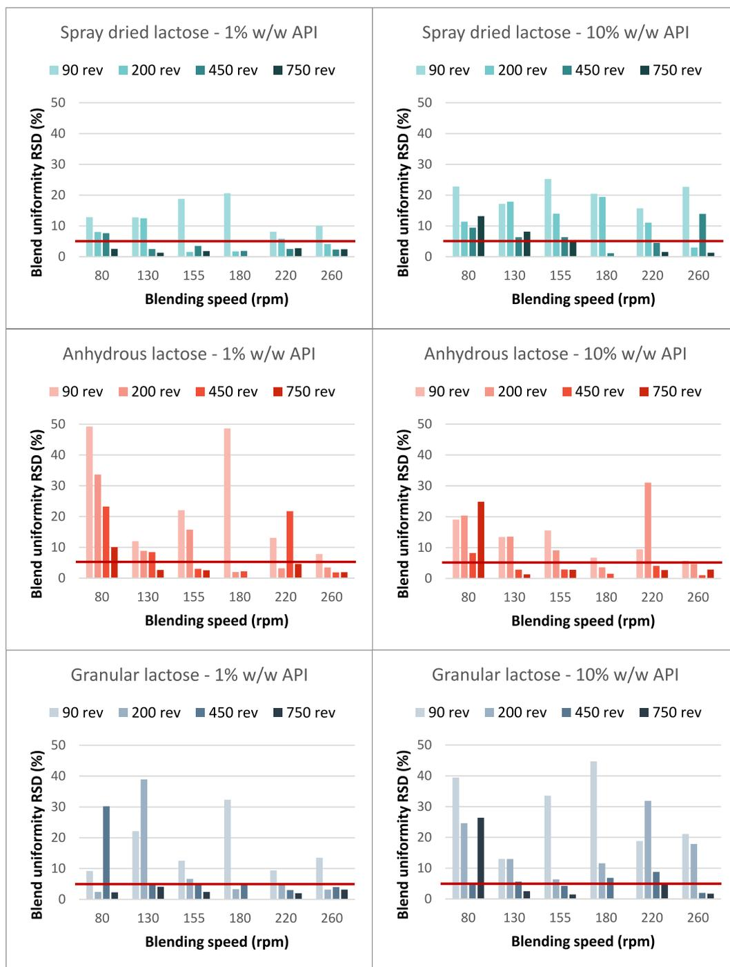
**Fig. 2.** Blend uniformity results for the six API-excipient blends based on three different lactose grades prepared at varying blender speeds at a fixed number of blender revolutions. Graphs show the relative standard deviation of the API concentration of the samples analyzed for each blend.
