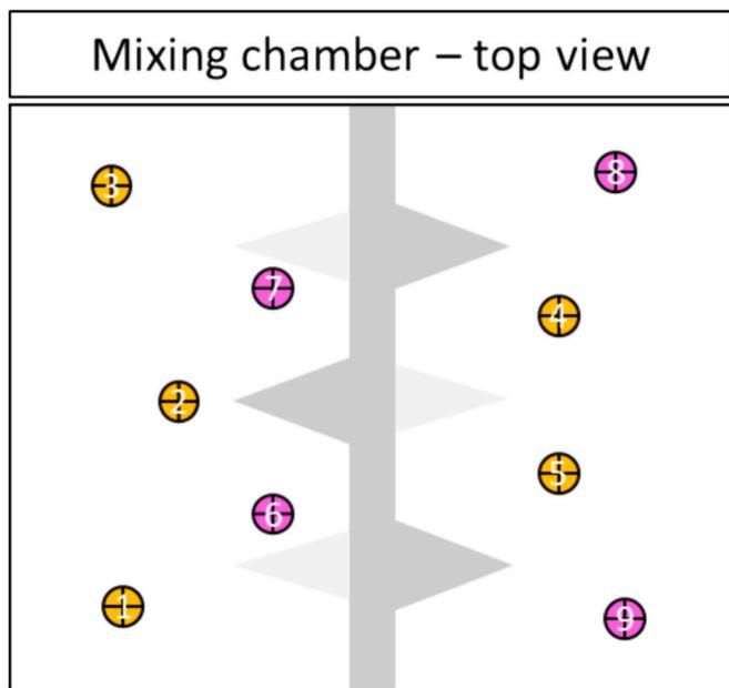
**Fig. 1.** Schematic overview of the sampling plan used for extracting samples from the mini-blender for blend uniformity analysis. The yellow dots represent sampling spots from the top half of the powder bed and purple dots represent sampling spots from the bottom half of the powder bed. Gray triangles represent the mixing blades of the mini-blender. (For interpretation of the references to colour in this figure legend, the reader is referred to the web version of this article.)
