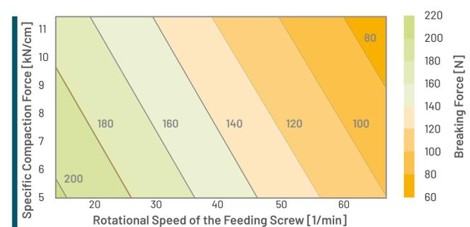
Fig. 3 Contourplot of the breaking force [N] of tablets (relating to a tableting compaction force of 10 kN). RCDG material of SMCC:DCP was produced at a constant roll speed (8 min<sup>-1</sup>), varying specific compaction forces and screw speeds
