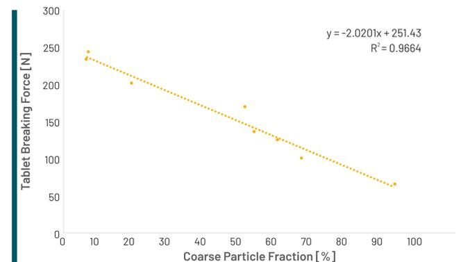
Fig. 1 Correlation between the coarse sieve fraction and the breaking strength of the SMCC:DCP (3:1) tablets (tablet weight 500 mg, compaction force 10 kN)
