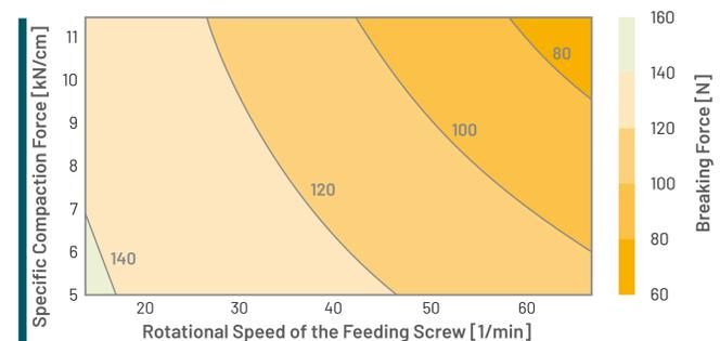
Fig. 2 Contourplot of the breaking force [N] of tablets (relating to a tableting compaction force of 10 kN). RCDG material of MCC:DCP was produced at a constant roll speed (8 min<sup>-1</sup>), varying specific compaction forces and screw speeds
