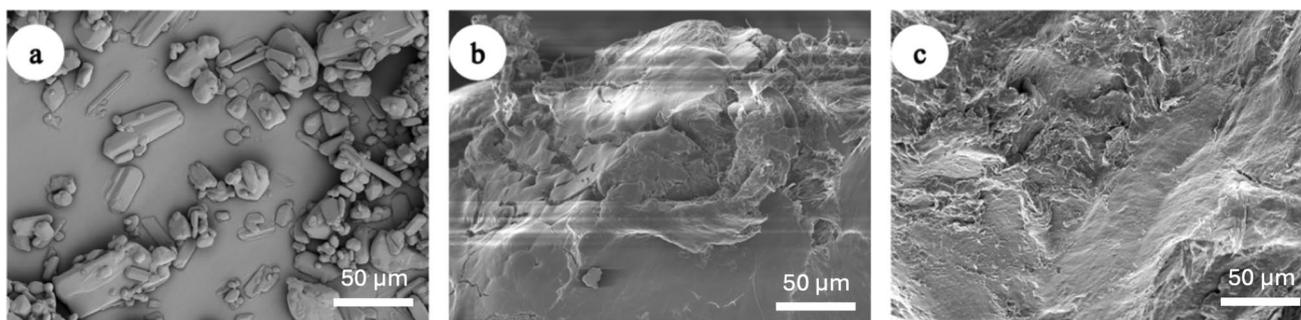
**Fig. 7** Scanning Electron Microscopic images of **a** Pure CBD, **b** F1V, and **c** F2V
