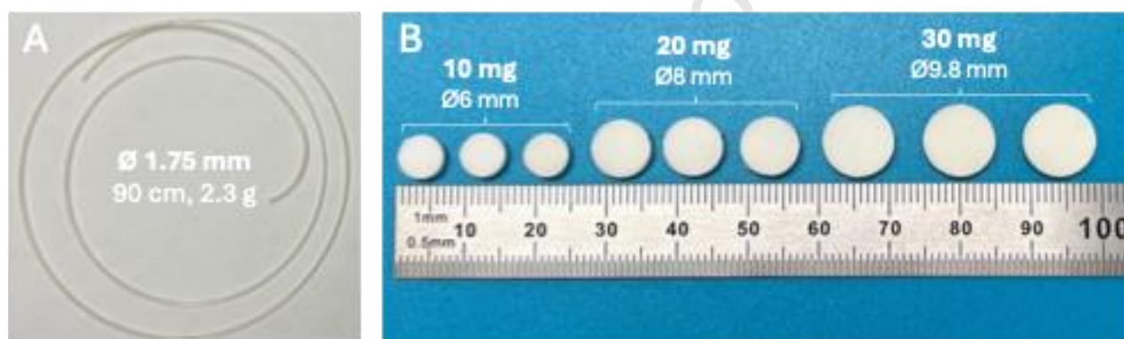
Figure 2: A) Image of VCM produced pharma-ink (filament) containing tamoxifen and B) image of three printlets of 10 mg, 20 mg, and 30 mg tamoxifen base (left to right). Scale in mm.
