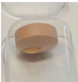
Fig. 3 Adalat® CR after 3 weeks of storage at accelerated conditions. A yellow watery drop is visible at the perforation of the membrane-controlled osmotic system
