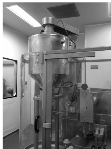
Figure 5: Feeding hopper and filling nozzle
