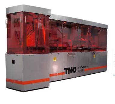
The TNO PrintValley 3D printing setup: a new approach to rapid 3D printing, employing a carrousel type-arrangement of building platforms passing underneath multiple printing heads in order to significantly speed up production. The setup can print several dozens of ODF size objects per second. This approach may be used for pharma as well in order to reach relevant production volumes.
