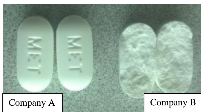
Figure 4.4: An example of capped metformin HCl tablets obtained from Company B’s API compare to un-capped tablets obtains from Company A’s API
