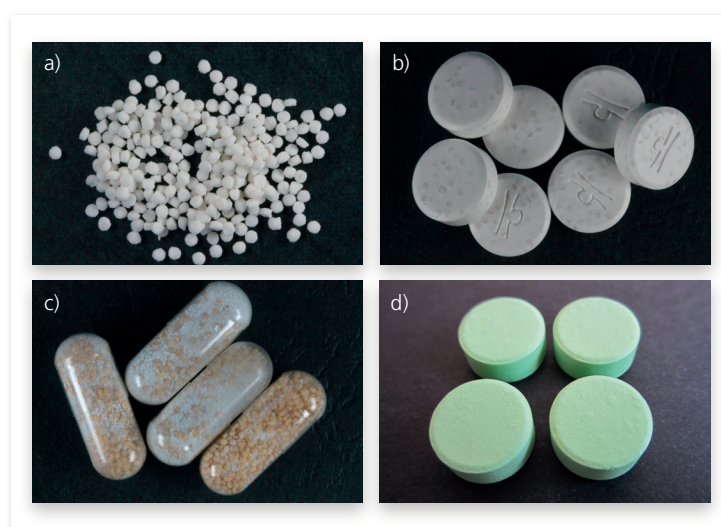
Figure 5) a) INTAC ® IR pellets; b) IR tablet manufactured on rotary press; c) IR fixed-dose combination capsule (pellets colored for illustration purpose only); d) IR tablet with non-functional cosmetic coating (Wening et al.) 28)
