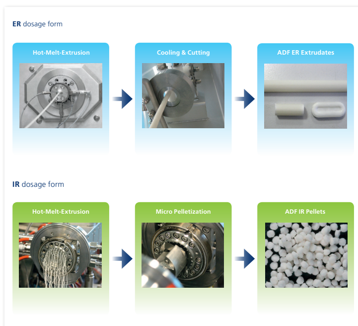
Figure 4) Process overview of INTAC ® hot-melt extrusion manufacturing concept for ER and IR products (taken from Wening et al.) 28)
