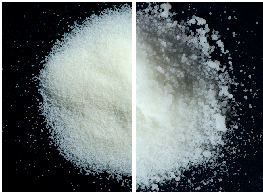
Figure 1: Next-generation powder manufacturing technologies (left) can provide narrow particle size distributions while offering taste-masking and controlled release in a single step, which overcomes limitations provided by traditional powder manufacturing methods (right).
