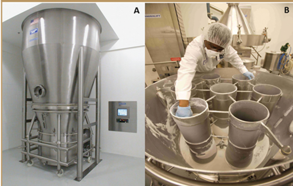
A) Fluid-Bed Coater & B) Wurster Setup for Taste-Masking
