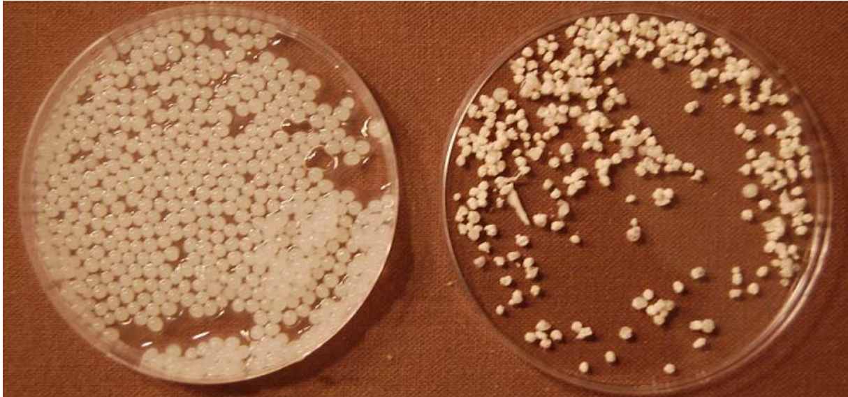
Figure 15 Microcapsules before drying (left) and after drying (right)
