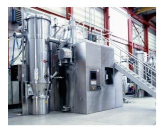
Finally, the combination of a high shear granulator with a fluid bed dryer combines the various options above, often in a highly space efficient manner. In addition, the close coupling often allows more integration before the system leaves
