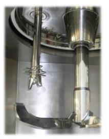
A typical high shear granulator is shown to the right, consisting of a main impeller on the bottom of the processing chamber and a chopper located higher up in the chamber. The main drive shaft can enter through the top (see photo on left) or bottom of the processing chamber but in both cases the impeller imparts shear energy by moving the product along
