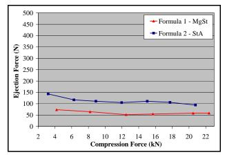
**Figure 1. Ejection Force Profile**
