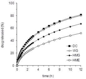
Figure 4: Effect of preparation method on niacin release.
